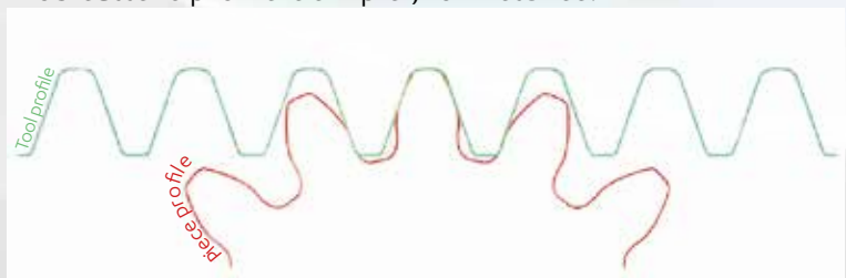
Hob cutter's profile is simpler, for instance:
